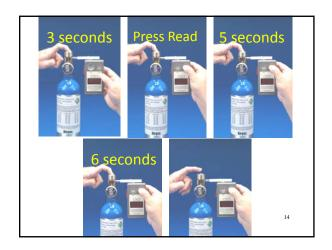
**Step 10: Adjust Setting** When the results are displayed adjust the reading so that it matches your alcohol standard. Turn clockwise to increase the reading, and counterclockwise to decrease the reading.
