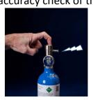
**Step 3: Determine Gas Value** by reviewing the elevation chart on the tank to calculate the alcohol concentration for the 0.038 tank at your elevation. The value can also be determined more easily by utilizing a True-Cal device.
